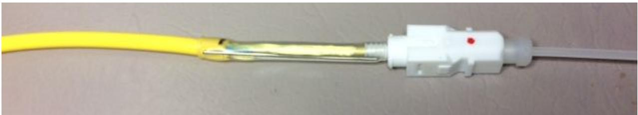
12. Slide SC components up fiber until reaching the spliced connector. Next, slide the rear boot up until snapped on the the back portion of the ferrule assembly. Tighten the threaded cap over nose of the rear housing. Slide the front shell over the dust cap. While ensuring that the red dot is up, snap the housing onto the connector. The red dot should be aligned with the housing key.
