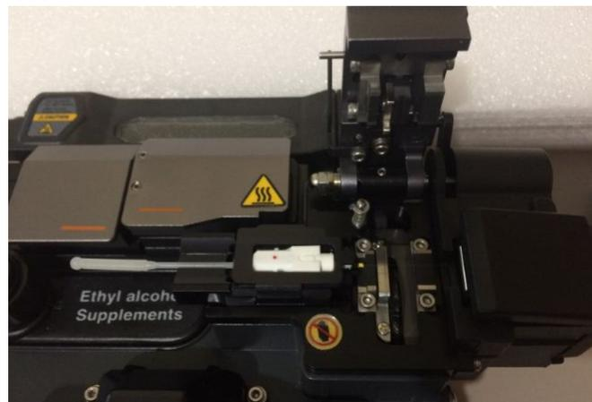
intermediate position. Door will actuate shut during cleaving operation as part of the disposal process. Forcing the door shut at this point WILL DAMAGE the door.
