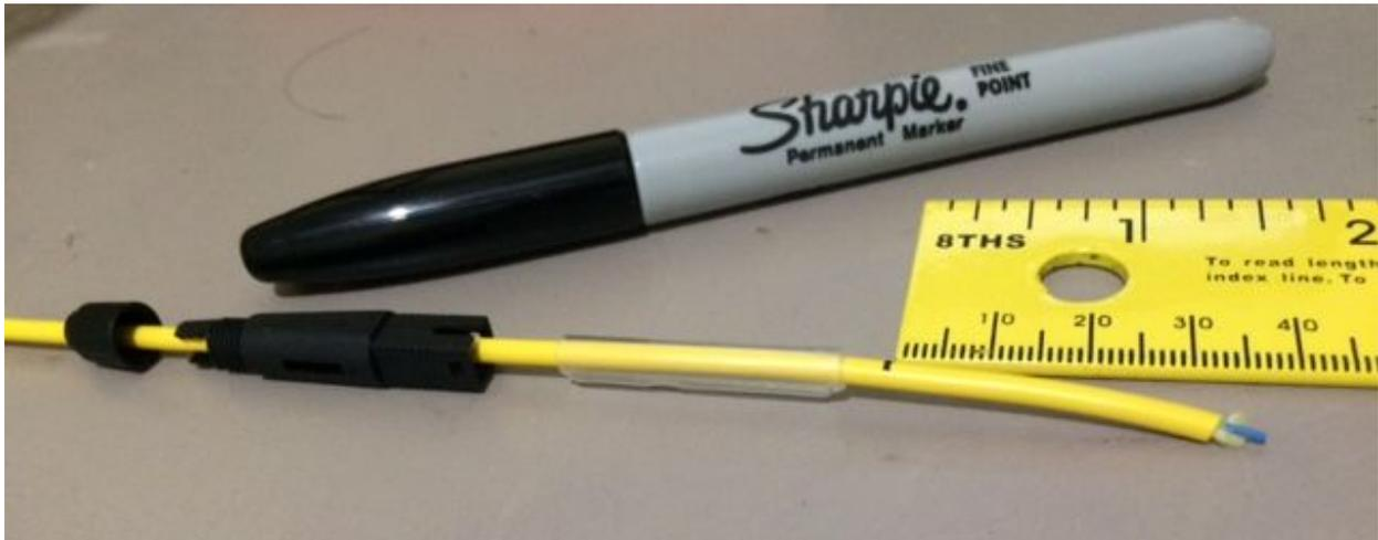
3. Using a hand stripper, remove the outer 3mm jacket from the mark outward.
